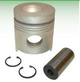
**41081** Piston Kit Early 7000 *17mm to top of first ring, 41080 is late* Bore size: 111.77mm
