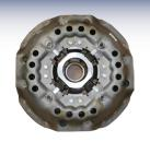
2937 Clutch Assembly Ford 4600 - 13" Synchro Transmission only Clutch Aligning Tool = 43121
