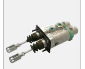
**42917** Brake Valve Booster New Holland T7030 T7040 OE Ref: 87315873
