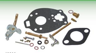
**48800** Carburettor Repair Kit Fordson 2N 8N 9N
