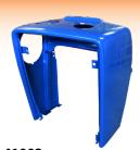
41003 Nose Cone Ford 5600 - 7600 with Dry AirFilter
