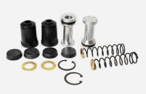
**4284** Repair Kit Ford TW Brake Master Cylinder
