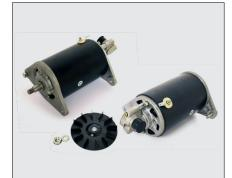
**41634** Ford 2000 - 7000 Dynamo Includes Tacho *Suitable for 11A & 22A Regulator Open Type* OE Ref: 3109419R91
