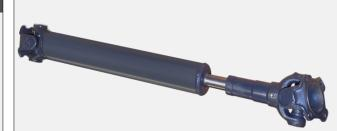
**43569** Driveshaft New Holland TM120 TM130 TM140 TM155 TM175 TM190 OE Ref: 87393883
