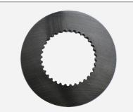
**43935** Hand Brake Disc T6030 - T6090 T7.170 - T7.210 TM130 TM120 TM140 TM155 *180mm x 105mm 4.5mm* OE Ref: 47127719
